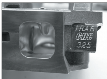
426-1RA6 CNC 325cc Intake Runner
